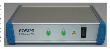
The sampling is done by using the internal clock or can be controlled by an external trigger signal to synchronise the measurements with other devices.
